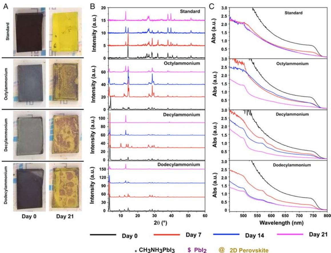
**Figure 5.** A) Photographs of the perovskite films showing the degradation patterns of perovskite films deposited over the planar substrate after 21 days of exposure to environmental conditions. B) XRD and C) UV-vis spectra of perovskite films deposited over the planar substrate, with and without the modification, at the beginning and after 7, 14, and 21 days of exposure to environmental conditions.
