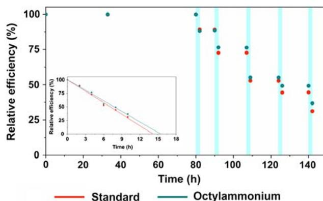
**Figure 7.** Efficiency loss related to the degradation of the device by exposing the devices to ambient temperature and humidity conditions.
