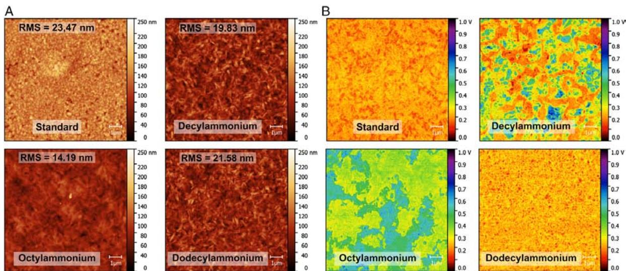
**Figure 2.** A) Atomic force microscopy images and B) Kelvin probe force microscopy image of the surface of perovskite films with and without the modification with octyl, decyl, and dodecylammonium chloride surfactants, respectively.
