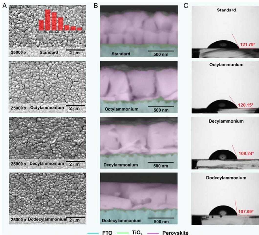
**Figure 1.** A) FEG-SEM images of the perovskite films deposited on planar  $\text{TiO}_2$  substrate with and without surfactant modification with octyl, decyl, and dodecylammonium chlorides. The inset displays the crystallite size distribution of standard perovskite films. B) FEG-SEM cross-section images of perovskite films deposited on the planar substrate. C) Contact angle measurements between water drops and the surface of perovskite films on planar substrates.
