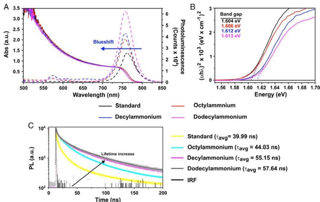
**Figure 4.** A) Normalized UV–vis and PL spectra and B) Tauc plots of the perovskite films deposited on planar TiO<sub>2</sub> substrate with and without modification. C) PL decay of different perovskite films with the average lifetimes.
