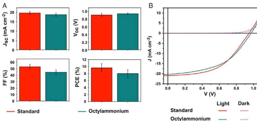
**Figure 6.** A) Devices parameters ( $J_{sc}$ ,  $V_{oc}$ , FF, and PCE) of solar cells prepared without and with the modification with octylammonium chloride. B)  $J \times V$  curve of the champion's devices.
