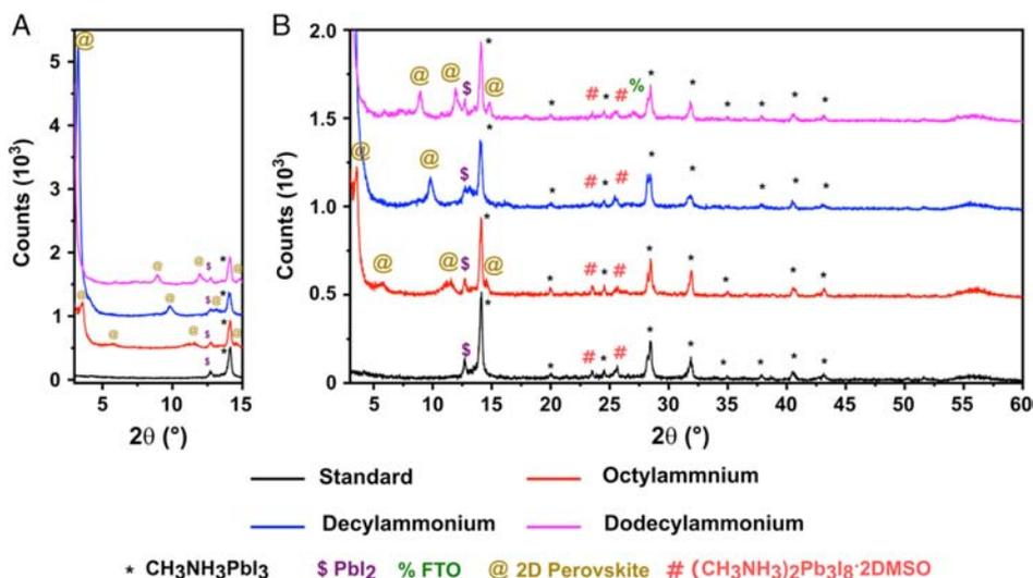
**Figure 3.** XRD patterns of  $\text{CH}_3\text{NH}_3\text{PbI}_3$  films deposited over planar  $\text{TiO}_2$  substrate before and after the modification with the surfactants. Focus on 2θ A) from  $2.5^\circ$  to  $15^\circ$  and B) from  $3^\circ$  to  $60^\circ$ .
